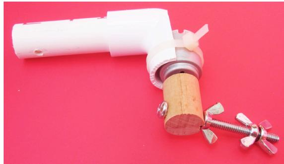
11. Attach the complete motor assembly shown in the previous photo to the masonite-wood platform by placing one of the small washers on the remaining machine screw and pushing the screw up from the bottom of the platform and through the two holes in the PVC pipe. Put the remaining small washer and remaining wing nut on the protruding end of the machine screw and tighten the wing nut to hold the motor assembly firmly in place. See photo below.
