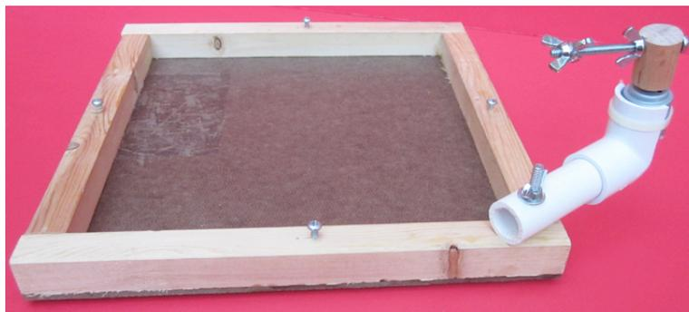
12. Lay the platform with motor assembly on the marbles in the caps on the base, and put a rubber band around each of the four corresponding pairs of screws. See photo below.
