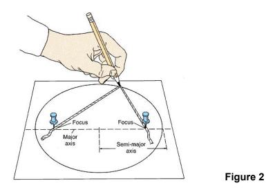
Measure the major axis (widest part) of the ellipse. Measure the distance between the pushpins. Calculate the eccentricity of the ellipse that you drew by using the following formula:
