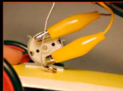
Connect motor. Connect the motor to the solar panels.
