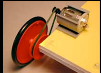
Motor and pulley mounted. Position the motor on the car body.
