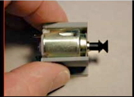
Motor assembly. The electric motor in its mounting clip.
