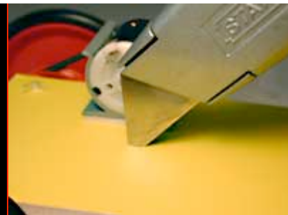
Slot cutting. Cut a slot for the paper fastener.
