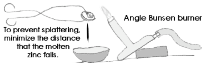
Figure 1: Melting zinc with a Bunsen burner
